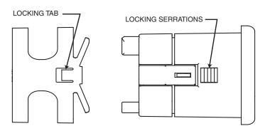
LOCKING TAB MUST ALIGN WITH LOCKING SERRATIONS
